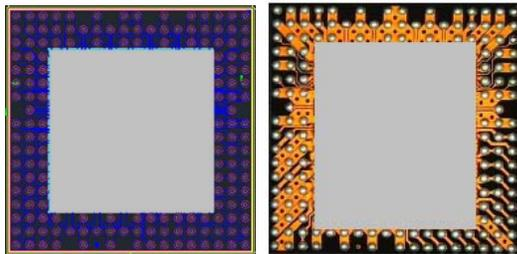
Figure 2. PKG drawing and micrograph of test vehicle of 9x9mm, 0.5mm pitch eWLB.
