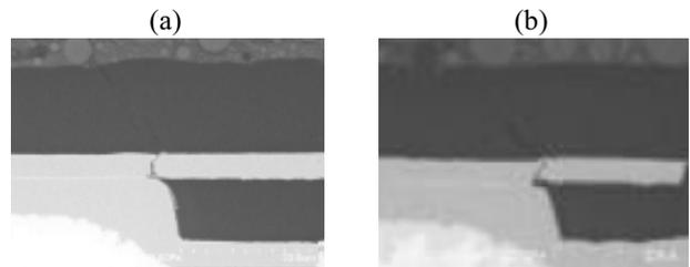
**Figure 8 . SEM micrographs of failure of DOE 4 (with UBM & NSMD)**
