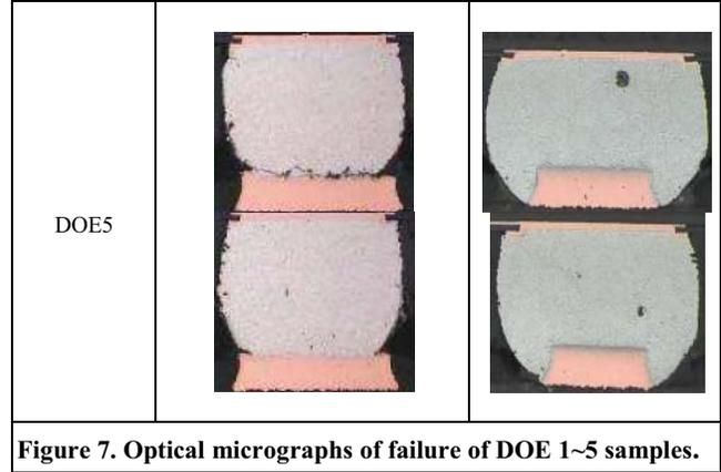
In this study, both DOE 4 and 5 UBM samples showed lower solder joint life cycle compared to non UBM samples. For UBM samples, SMD of DOE 4 and 5 showed solder fatigue failure in board side as shown in Fig. 7 but NSMD of DOE 4 and 5 did not have major solder fatigue cracks. After further failure analysis of SEM micrographs, the Cu metal pad was observed as broken in conventional WLCSP [17,18,19].
