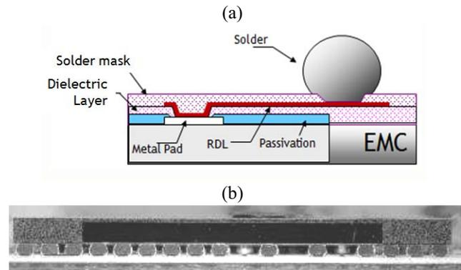
Figure 3. (a) stackup drawing of eWLB and (b) micrograph of cross-section of test vehicle as shown Table 1.
